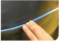
Use 3M<sup>TM</sup> Fine Line Masking Tape 471 in 3mm (06404) and 6mm (06405) for accurate masking and detailing.
