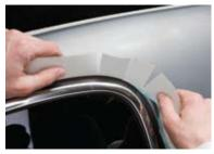
Use 3MTM Trim Masking Tape (06345/47/48/49) on windscreens and components to provide complete protection from overspray.
