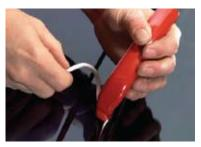
Use 3MTM Trim Lifting Cord (09529) under rubber mouldings to prevent a hard paint edge forming.
