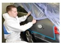
Use 3MTM Premium Clear masking film (80139/50366) to protect those area of the car not to be sprayed during the repair. One man application and clinging properties speed up masking times.
